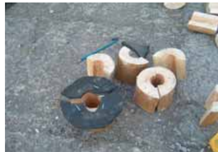
Swabbing tool under manufacturing by using wasted old tire and wooden materials
