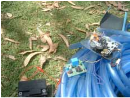
Left: Timer set by Radio Deck and E-K Japan (PU-2705) Right: Tested depth: 120m (battery is in plastic bag)
