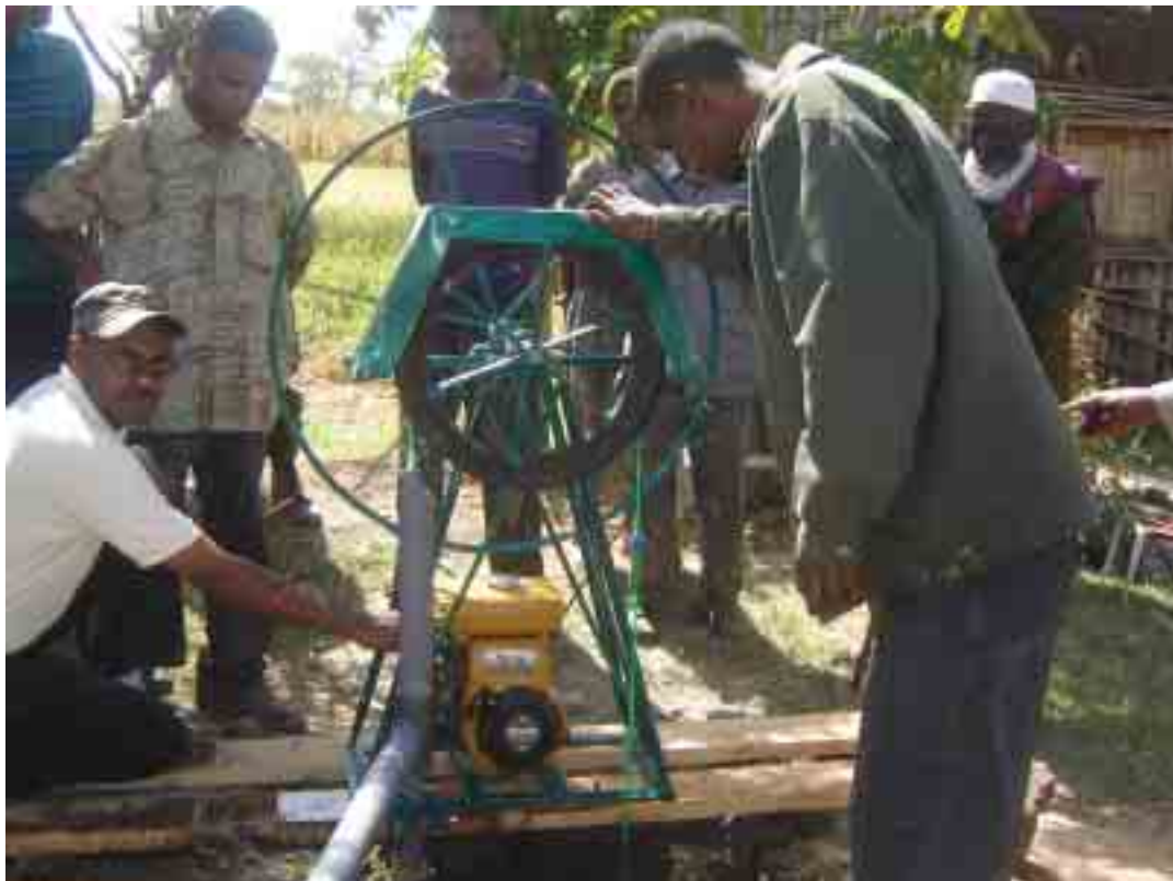
Figure 62: Motorized (diesel motor) rope pump demonstration.
